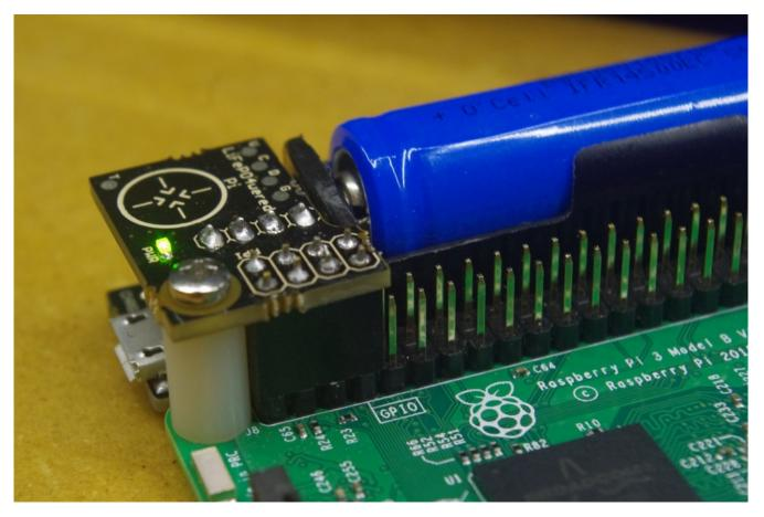
There is also a version available with stackable 40-pin header, which allows the user to install the  $LiFePO_4wered/Pi^{TM}$  in combination with other HATs.
