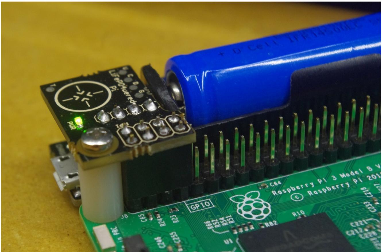
There is also a version available with stackable 40-pin header, which allows the user to install the LiFePO<sub>4</sub>wered/Pi™ in combination with other HATs.
